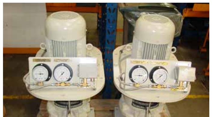
Shock Rated Engine Room Pump
