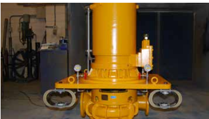
Shock Rated Engine Room Pump
